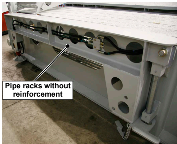
Figure 2: Pipe racks with and without reinforcement
